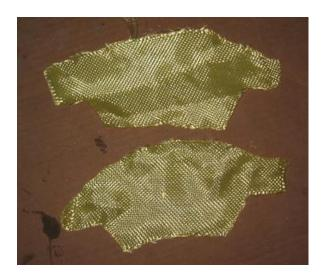
10. Wet out the underside of the deck and inside of the hip blocks with epoxy resin and add a first layer of carbon (or kevlar) resin saturated reinforcement.
